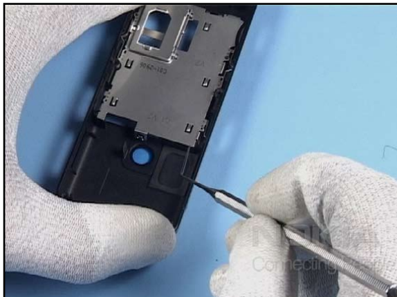
31. Release the shown metal snaps of the LABEL COVER ASSY with the dental pick.
