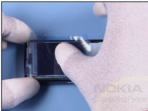
13. Cover the display with a film.
