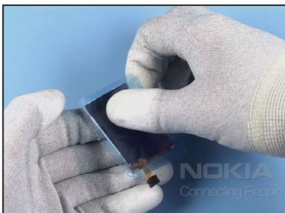
23. Cover the display with a film again.
