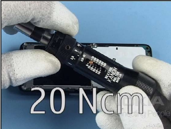
13. Set the correct torque.
